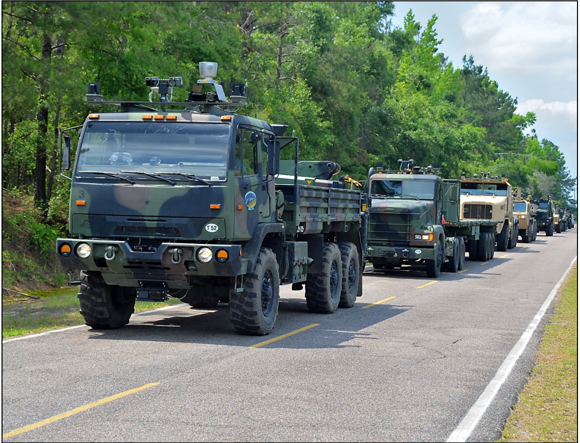
A convoy of driverless Army trucks makes its way through the Department of Energy's Savannah River Site in South Carolina, May 29, 2014. Photo Credit: U.S. Army Tank Automotive Research, Development and Engineering Center.
